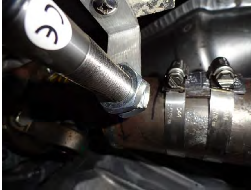
Figure 3.18 Tachometer and imbalance mass attached at the front driveshaft
