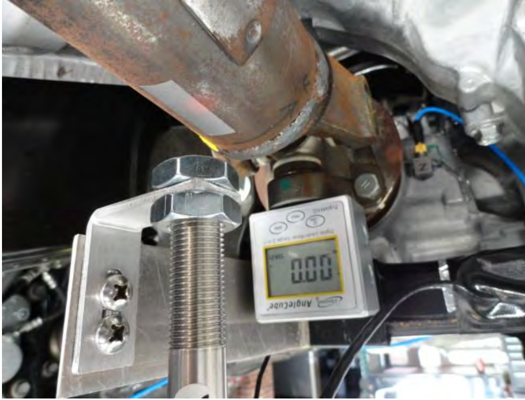
Figure 3.4 Plane A with a tachometer and reflecting strip is set as 0° angle
