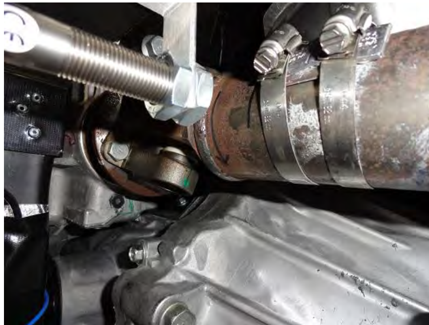
Figure 3.19 Front-axle plane and the tri-axial accelerometer position is pointed out
