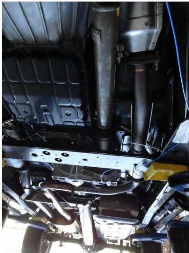
Figure 3.7 Front and rear drivelines, from underneath the truck.
