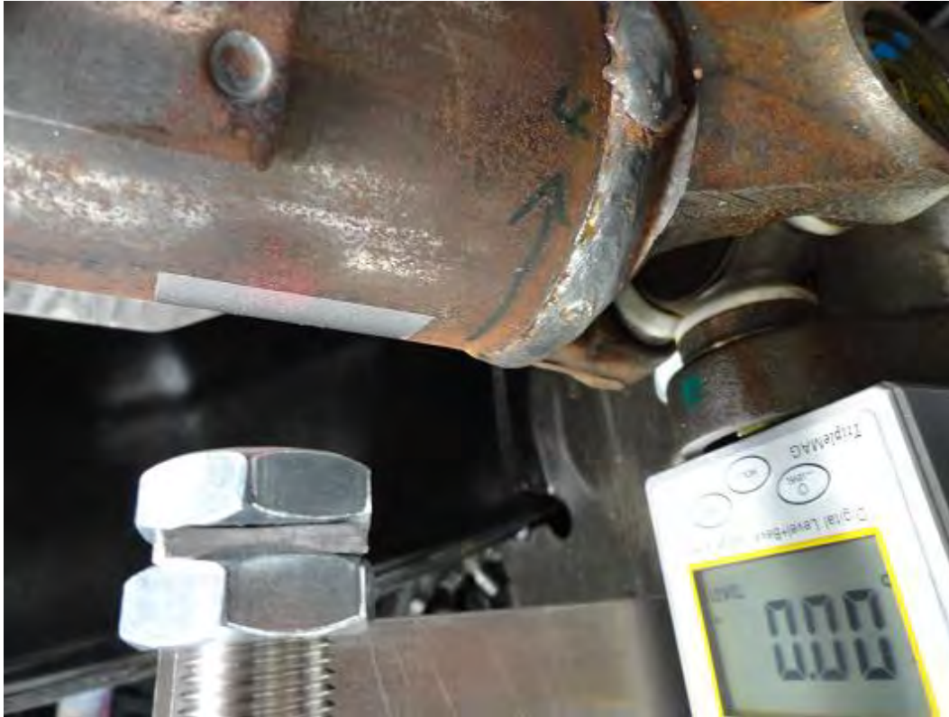
Figure 3.8 Front driveline axle plane with tachometer and reflective tape
