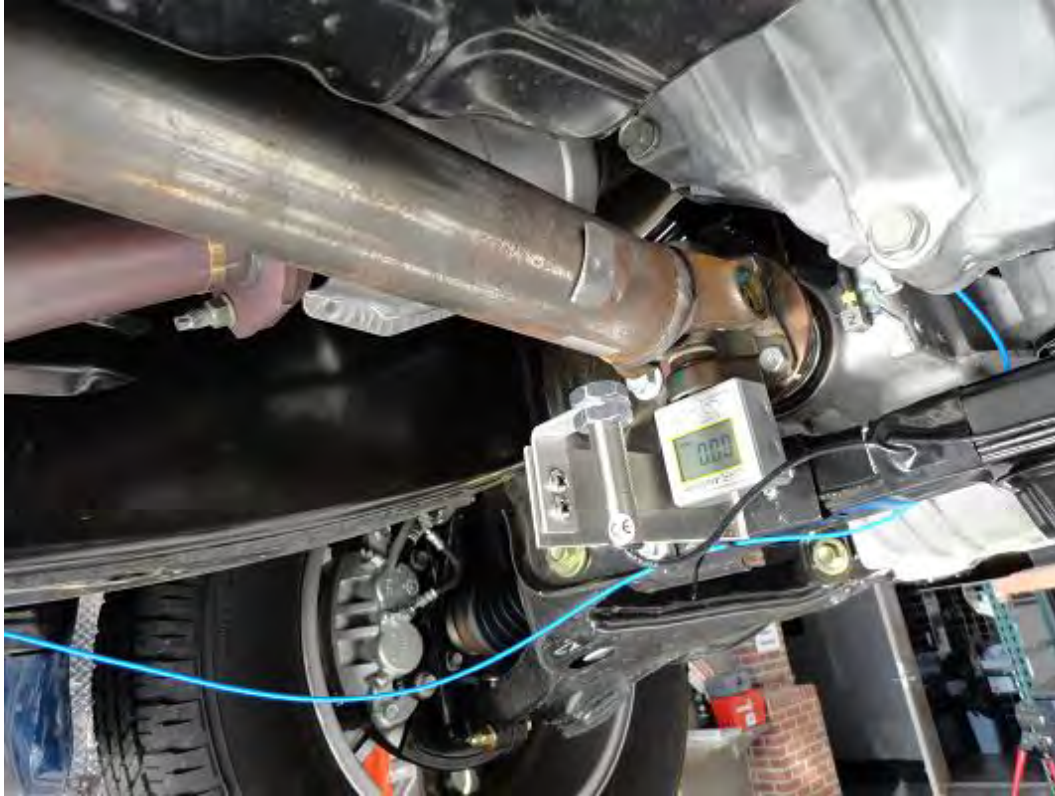
Figure 3.9 Front driveline axle plane with a tri-axial accelerometer.
