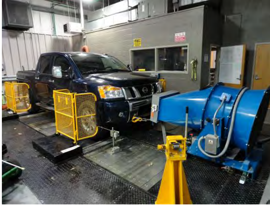
Figure 3.12 Truck tested on dynamometer
